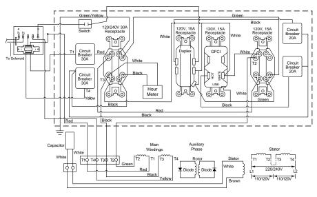
Figure 22 - Wiring Diagram, Model PGH7500IE
